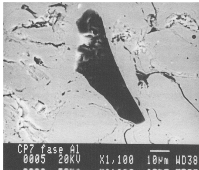
Fig. 9 Cross section of a mixed metal-ceramic coating showing an aluminum-containing phase (dark area)
